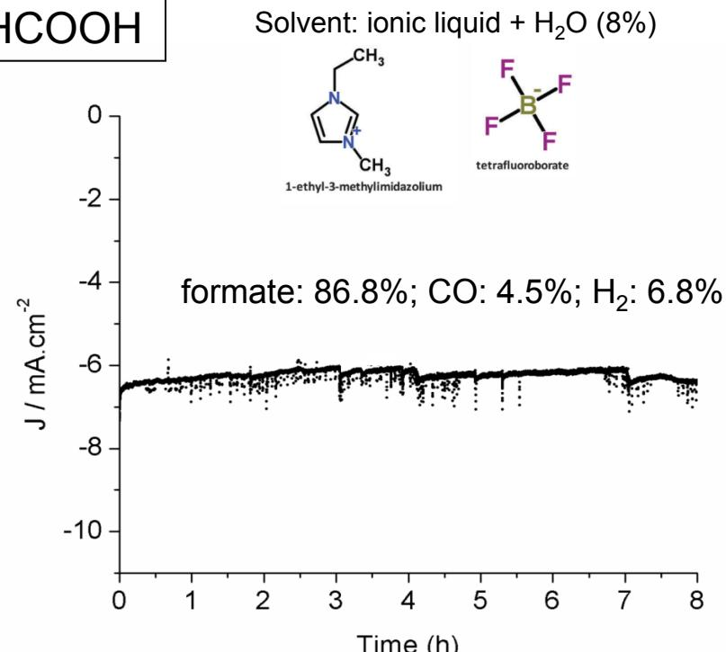
CPE of  $\text{CO}_2$  at -1.55 V vs  $\text{Fc}^+/\text{Fc}^0$
