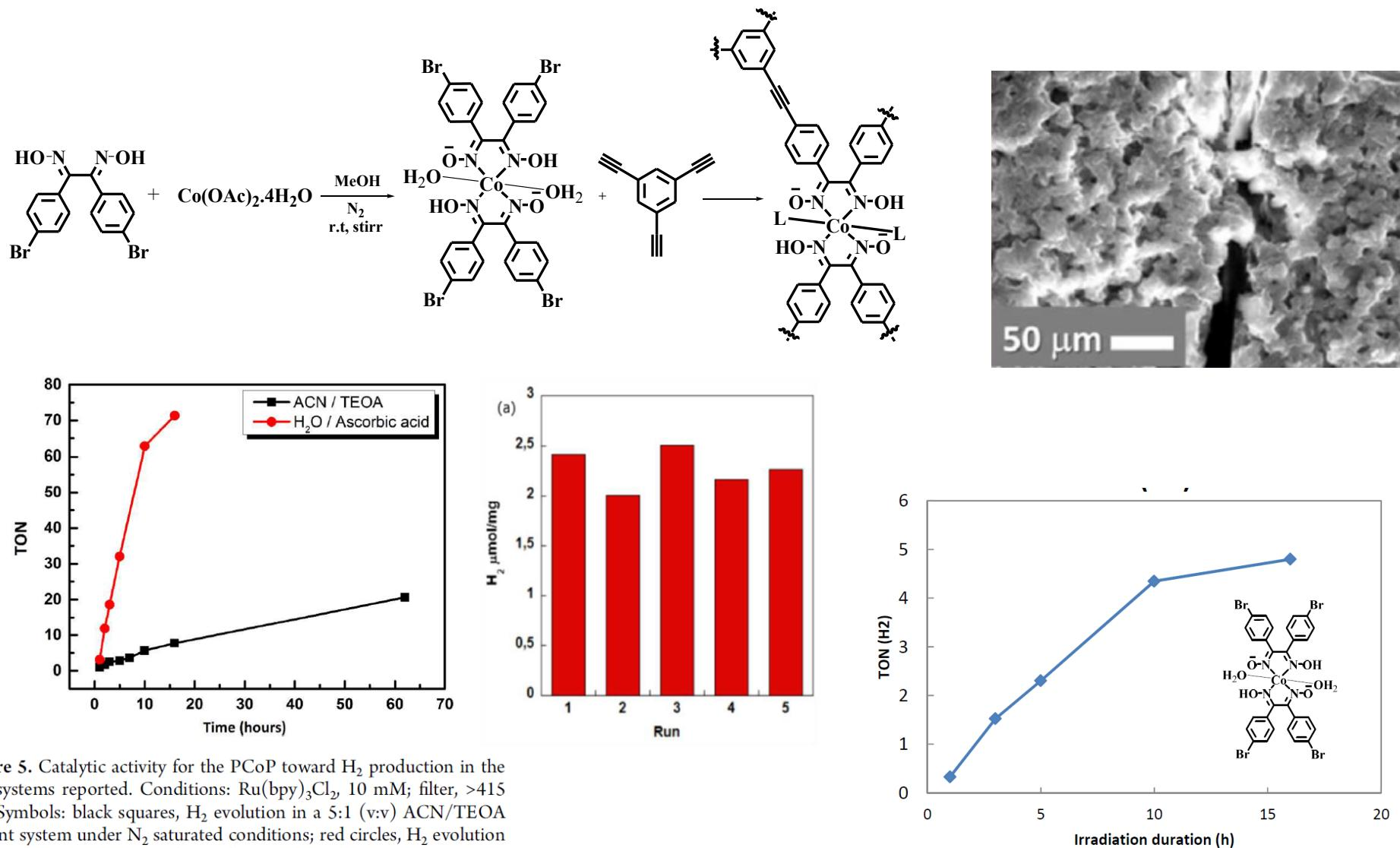
**Figure 5.** Catalytic activity for the PCoP toward  $\text{H}_2$  production in the two systems reported. Conditions:  $\text{Ru(bpy)}_3\text{Cl}_2$ , 10 mM; filter,  $>415$  nm. Symbols: black squares,  $\text{H}_2$  evolution in a 5:1 (v:v) ACN/TEOA solvent system under  $\text{N}_2$  saturated conditions; red circles,  $\text{H}_2$  evolution in an  $\text{H}_2\text{O}$ /ascorbic acid (0.1 M) pH 4 solvent system under  $\text{N}_2$  saturated conditions.
