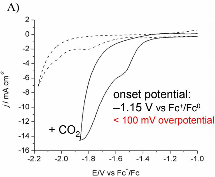
CVs on a modified Cu electrode
